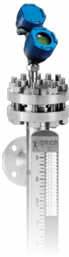
Orion Instrument's Aurora® MLI combines a conventional float-based MLI technology with the Eclipse® Guided Wave Radar transmitter. These devices operate seamlessly to provide a continuous 4-20mA & HART output and visual indication. The result is true level measurement redundancy in a single chamber.
